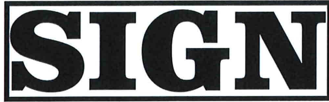
Illustration 7 Sign Surface area equals the smallest rectangle surrounding any writing or symbols
